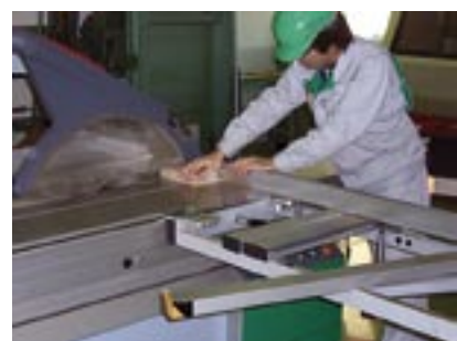
Sawing on a table saw, v, = handfeed, RPM = 4700 1/min.
